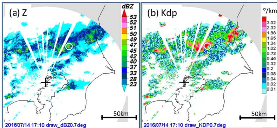
**Fig. 11 PPI plots of (a) reflectivity and (b) Kdp as observed using the Haneda DRAW with an elevation angle of  $0.7^\circ$  at 1710 JST on 14 July 2016. The black crosses and white circles indicate the locations of the Haneda DRAW and the Tateno site, respectively.**
