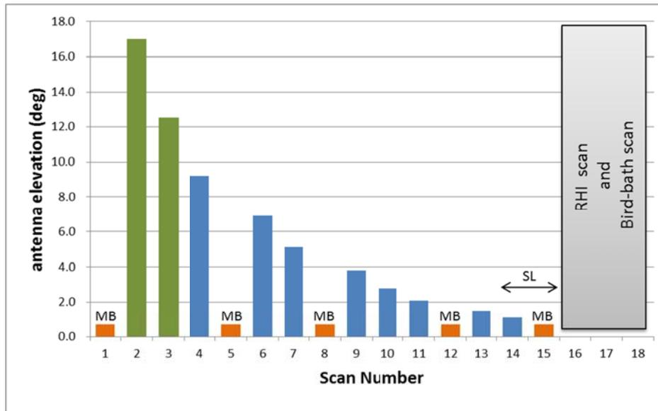
**Fig. 4 Five-minute antenna scan sequence**
