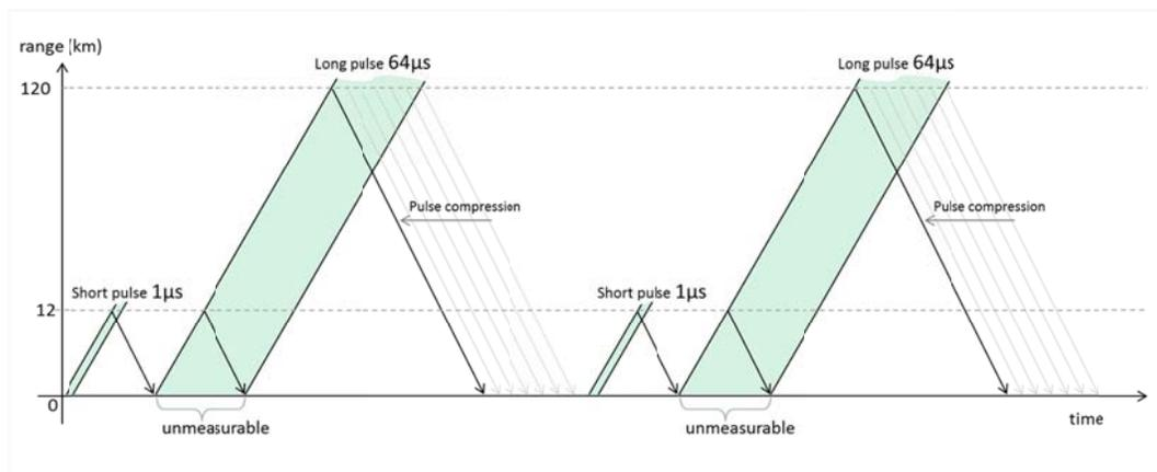
**Fig. 5 Relationship between pulse width and measurable area**
