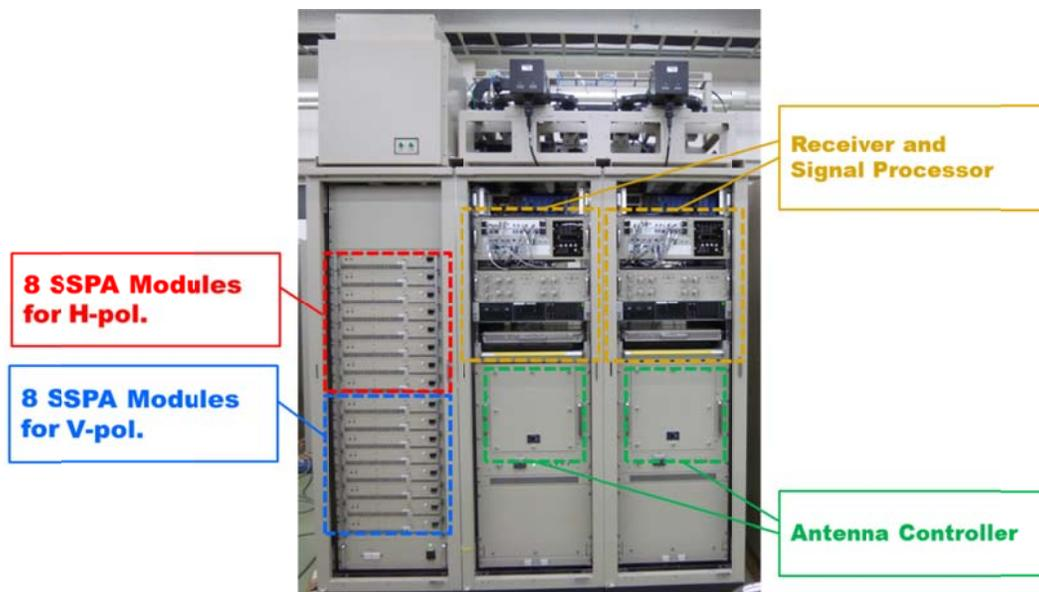
**Fig. 8** Transmitter, receiver, signal processor and antenna controller
