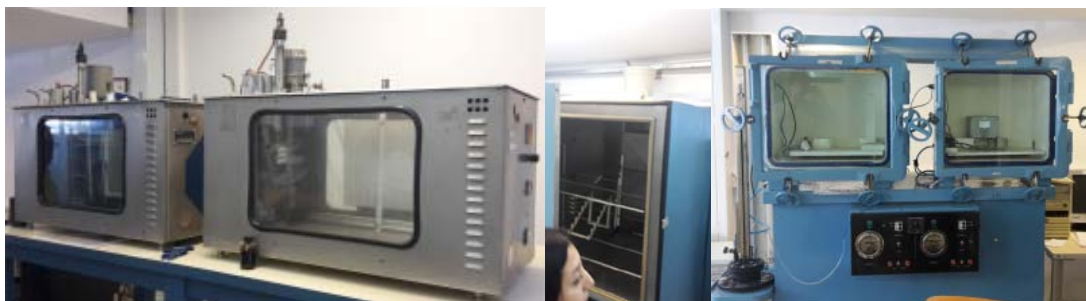
Figure 2: Calibration bath, climatic chamber, and pressure chamber.
