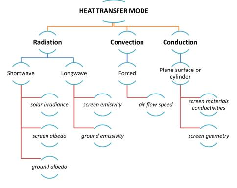
Figure 2. Ambient parameters contributing to heat transfer inside a meteorological shelter
