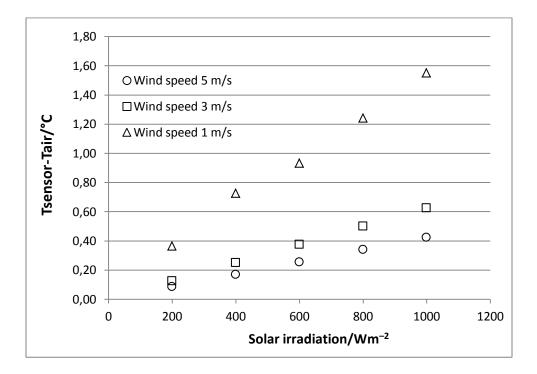
Figure 7. Temperature difference of the air inside the shield and surrounding air for different solar irradiations at different wind speeds
