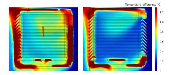
**Figure 5.** Temperature difference of the air inside the shield and surrounding air. Left: the plane cutting through the thermometer center (behind the door frame). Right: the plane located 250 mm to the left of the thermometer (behind the door louvers).
