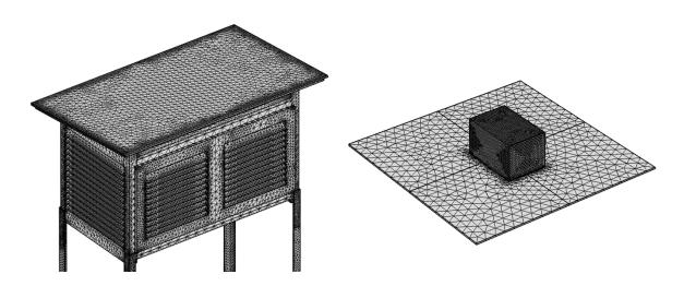
Figure 3. Screen and domain mesh.
