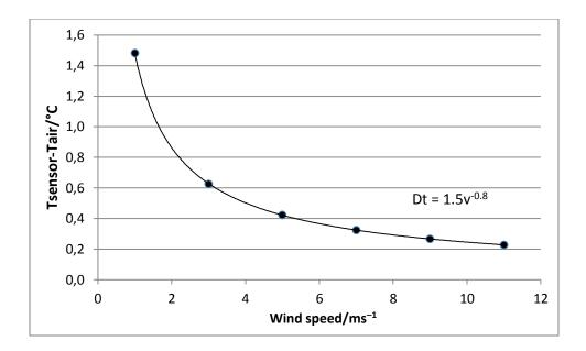
**Figure 6.** Temperature difference of the air inside the shield and surrounding air for different wind speed at maximum solar irradiation (1000 Wm<sup>-2</sup>).
